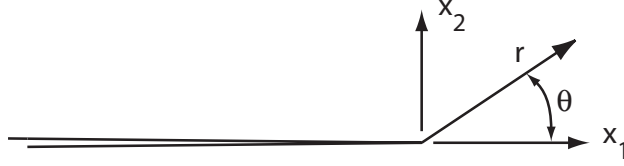
Figure 2.3: Semi-infinite crack in an infinite body. For clarity the crack is depicted with a small, but finite opening angle, actual problem is for a crack with no opening angle.
