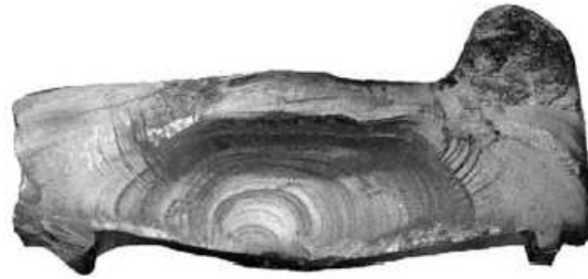
Figure 1.2: Fracture surface of broken ICE train wheel tire.
